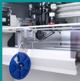
Intelligent feeders in all common sizes. Component spectrum from 01005 to 100x150 mm, component height up to 15mm
