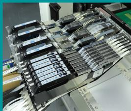
CANBUS connects all the modules working throughout the feeder controlling, so that they can work together to run effectively, more intelligence and fewer wires.
